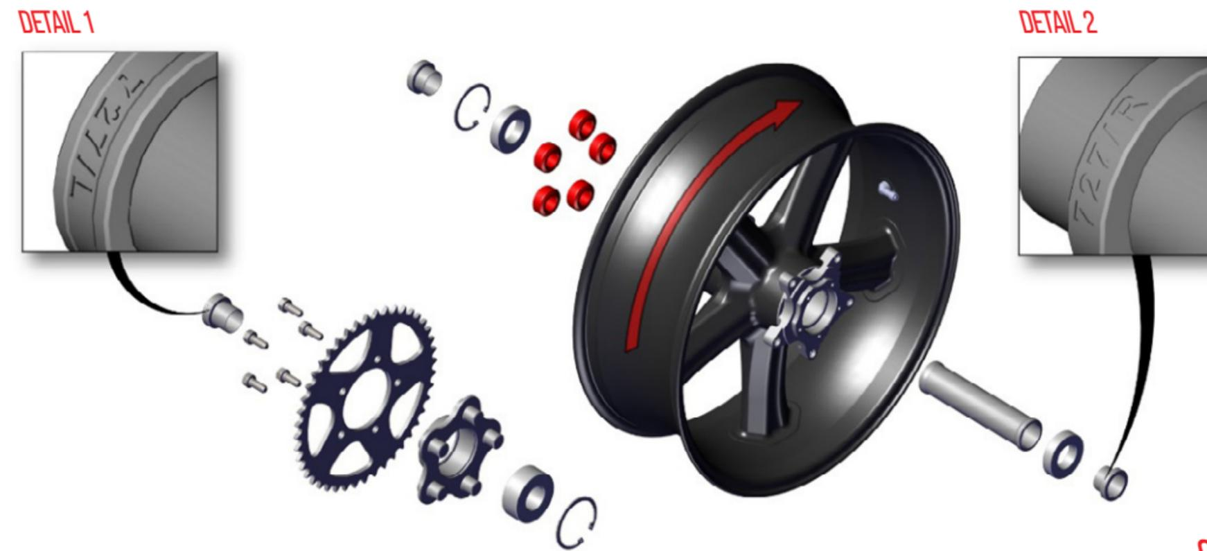
**FIGURE 3:** ASSEMBLY OF REAR CONVEX BOOST WHEEL WITH ACCESSORIES
