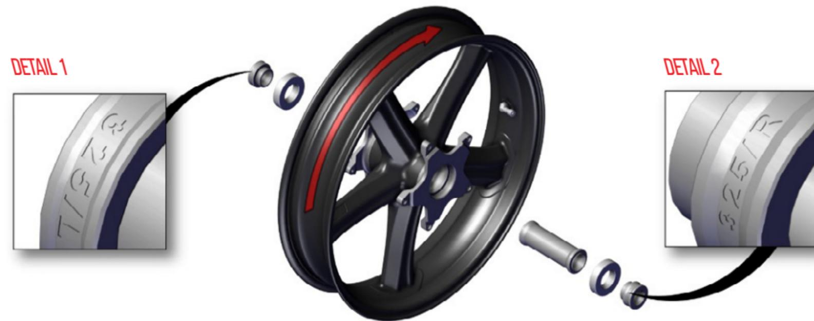
FIGURE 2: ASSEMBLY OF REAR SYMMETRIC BOOST WHEEL WITH ACCESSORIES
