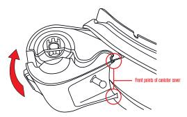
10. Continue pulling the film across to the other side. Be sure the top edge of the film stays between the mud visor and lens. Wrap the tape around the axle in the right side canister using the sticky side.
