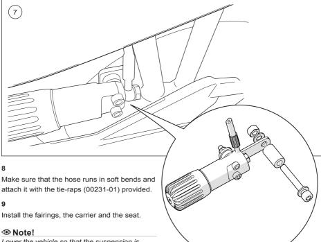
Lower the vehicle so that the suspension is slightly compressed before tightening the screws.
