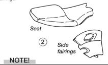
The screws holding the fairings are of different lengths. Make sure to return them to the correct position.
