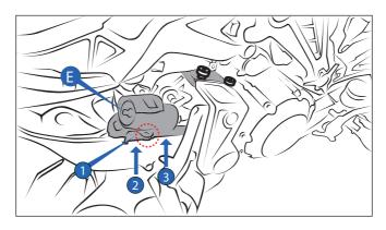
7. Remove the heat shield © by loosening the screws ①②③.
