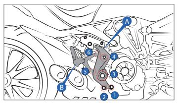
9. Uninstall the standard shock absorber by loosening the upper and lower mounting screws ①②.
