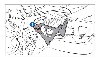
5 Remove the left side plate by loosening the screws  $\bigcirc \bigcirc \bigcirc \bigcirc \bigcirc \bigcirc \bigcirc$
