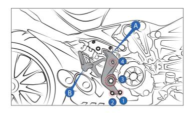
7. Remove the heat shield © by loosening the screws ①②③
