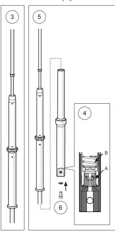
threadlocker and tightening torque. Install bottom bolt and washer. Use tool 8 mm allen key to tighten bottom bolt.
