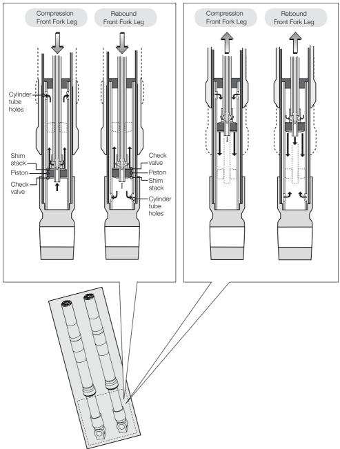
Fig. 4 - Front Fork Oil Flow Compression Movement
