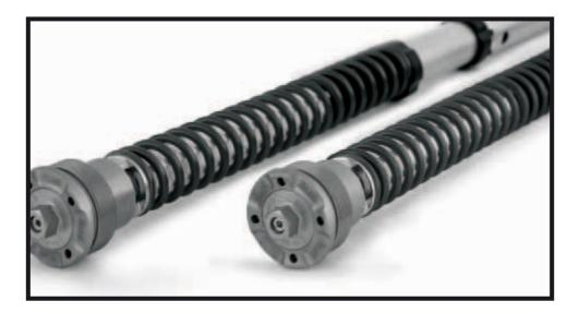
The front fork cartridge kit is divided into one compression cartridge and one rebound cartridge. The compression cartridge is installed in the left front fork leg and the rebound cartridge in the right front fork leg. Marked at the top cap is "COMP" for compression adjustment and "REB" for rebound adjustment (Fig. 1).
