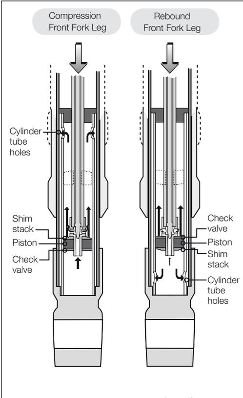
Fig. 5 - Front Fork Oil Flow Rebound Movement
