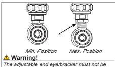
threaded out more than that the groove is fully visible beneath the lock nut. This is maximum length. After adjusting, make sure that the lock nut is tightened (30Nm).
