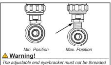
The adjustable end eye/bracket must not be threaded out more than that the groove is fully visible beneath the lock nut. This is maximum length. After adjusting, make sure that the lock nut is tightened (30Nm).
