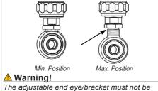
I he adjustable end eye/bracket must not be threaded out more than that the groove is fully visible beneath the lock nut. This is maximum length. After adjusting, make sure that the lock nut is tightened (30Nm).
