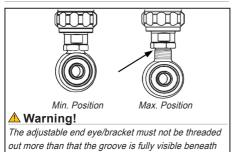
the lock nut. This is maximum length. After adjusting,
