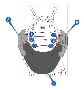
4 Remove the battery cover  $\bar{\mathbb{D}}$  by loosening the screws  $\bar{\mathbb{D}} \, \bar{\mathbb{Q}} \, \bar{\mathbb{G}}$  .
