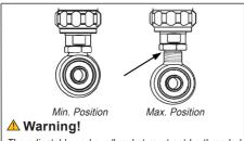
The adjustable end eye/bracket must not be threaded out more than that the groove is fully visible beneath the lock nut. This is maximum length. After adjusting, make sure that the lock nut is tightened (30Nm).
