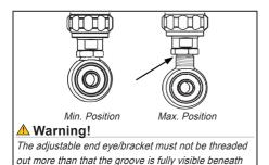
the lock nut. This is maximum length. After adjusting,
