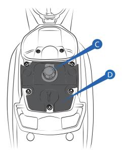
Remove the upper fairing  $\stackrel{\circ}{\mathbb{E}}$  by loosening the screws  $\stackrel{\circ}{\mathbb{S}}$ .
