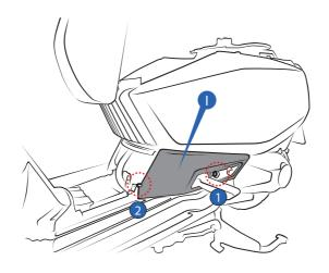
8 Remove the upper center fairing  ${\Bbb J}$  by loosening the screws  ${\Bbb S} { \Bbb A}.$  Repeat the operation on the opposite side.
