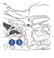
3. Remove the seat (B) by using the key unlock.
