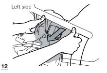
Remove the original shock absorber downwards.
