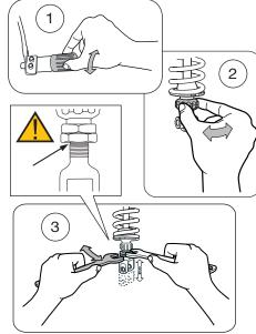
upper nut with one hand and at the same time loosen the lock nut (lower nut). Turn the end eye/ bracket to the desired length. Lock the lock nut. Tightening torque: 40 Nm
