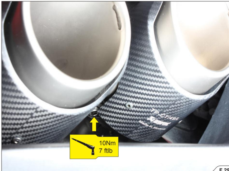
9. Reinstall all dismantled stock parts; check the vehicle manufacturer manual for correct procedures and tightening torques (F 30).
