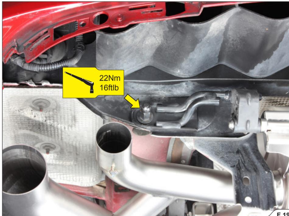
4. Align (lengthwise) the muffler's outlets by adjusting the marked joints and tighten the clamps to the specified torque (**F 20**).
