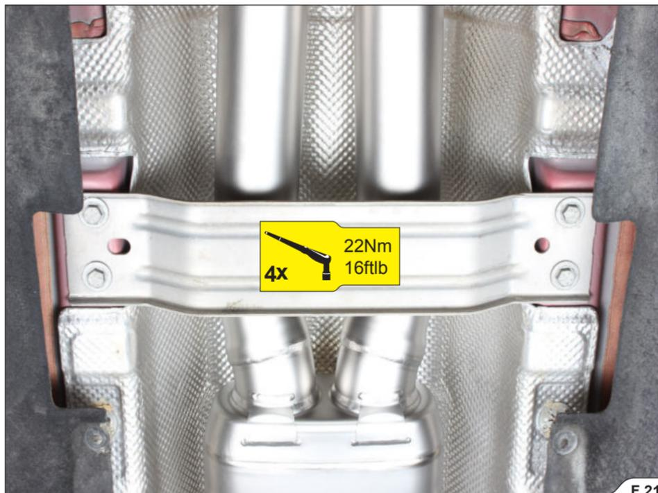
6. By rotating the front pipes, adjust the exhaust system (heightwise), so the middle muffler is in line with chassis reinforcement, then tighten the marked clamps to the specified torque (F 22, 23, 24).
