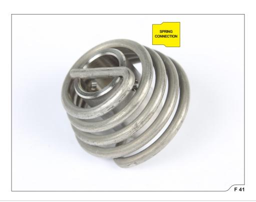
IMPORTANT: make sure, that spring connections seat correctly into the valves' axle groves (F 42, 43)!
