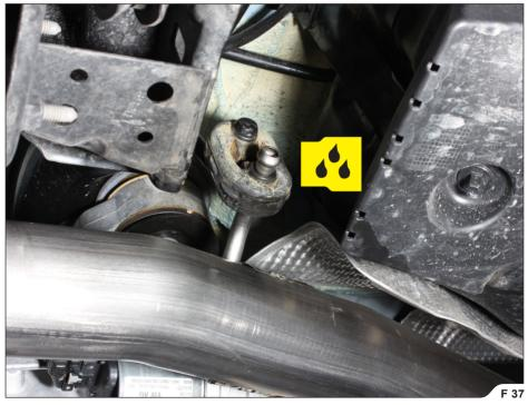
IMPORTANT: before tightening the clamps, adjust the muffler (length wise) in such a way, that clearance between muffler and rear axle carrier bolts is 40mm/1,57in (F 38, 39)!
