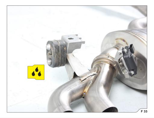
6. Carefully install the Akrapovič muffler onto the vehicle; tighten muffler's rubber brackets onto the chassis, redo the pipe's rubber brackets align the muffler in respect to the chassis (distance between muffler and rear axle carrier bolts should be 40mm/1,57in), slide the reduction bush with clamps all the way onto the muffler's inlet pipe and tighten the clamps to the specified torque (F 34, 35, 36, 37, 38, 39).
