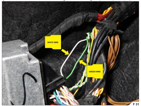
! IMPORTANT: test the Control Kit; in case it doesn't function correctly, use another pair of WHITE-GREEN wires for CAN sniffer (F 31, 32, 33).
