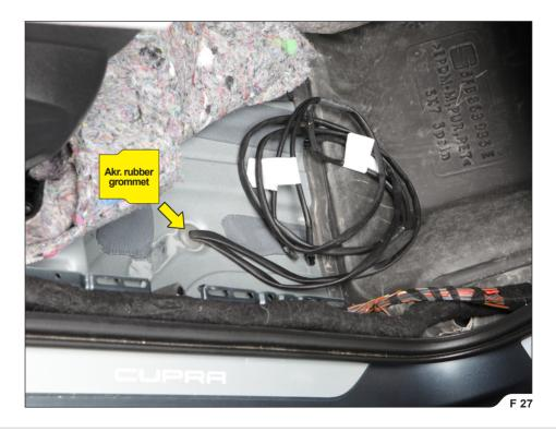
3. Install the Controller TNG and CAN sniffer as shown; carefully separate the **orange-brown** and **green** wires from the stock harness, unscrew the CAN sniffer's cover, lead the **orange-brown** and **green** wires through the CAN sniffer's wire grooves as shown, reinstall the cover, secure the components and harness (using tie wraps from Akrapovič installation kit) and reconnect the harness connectors to the Controller TNG (F 28, 29, 30, 31, 32, 33).
